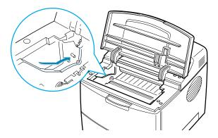
6 Grasp the handle and insert the cartridge in the printer until it snaps into place.
